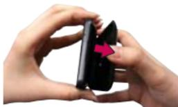
**1** Use the fingertip cutout at the bottom of the phone to remove the battery cover.
