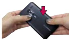
**3** Place the battery cover over the battery compartment, then press it downward until it clicks into place.
