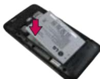
**2** Align the battery contacts with the terminals in the battery compartment and push the battery down until it clicks into place.
