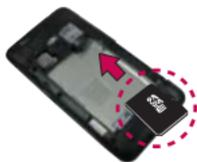
**NOTE** The microSD card can be easily damaged by improper operation. Please be careful when inserting, removing or handling it.
