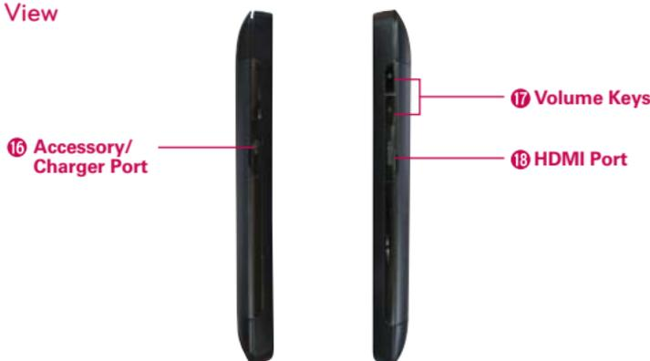
16. **Accessory/Charger Port** Allows you to connect the phone charger, USB cable, or other compatible accessories.
