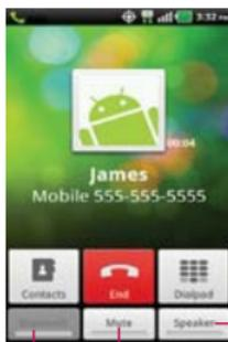
Touch to turn the speakerphone on or off. The Speaker Key lights up to indicate that the speakerphone is on.
